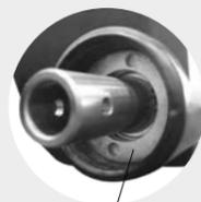
Bearing housing fitted with hard metal crown to remove bearing and shaft stress and in turn, any wear on the aluminium tube.
